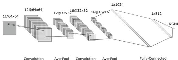
**Fig. 1:** Structure of the Convolutional Neural Network used to blindly predict NGMI.
