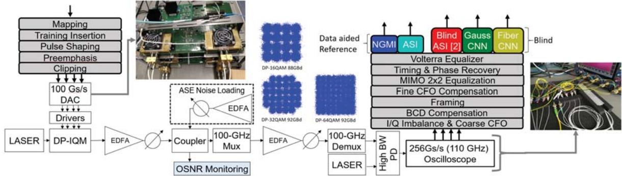
Fig. 2: Measurement setup including TX and Rx DSP with Blind GMI Monitoring
